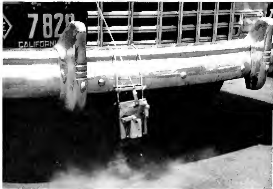
Double cartridge braking detonator. Using this bumper-mounted brake detonator a driver's reaction time and stopping distance are determined by cartridge fired chalk marks on the pavement.
